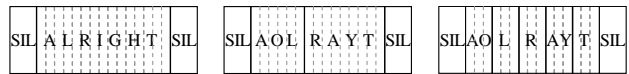
Figure 1: The different sub-word division methods: word model (left hand side), syllabication (mid) and phoneme based division (right hand side); dashed lines correspond to HMM states.
